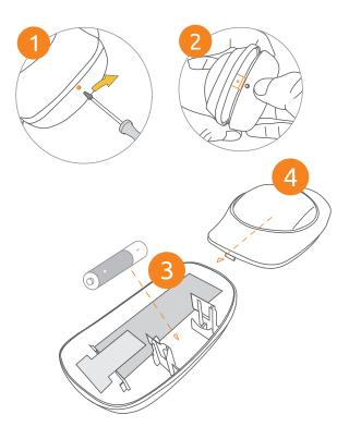
To remove the cover, release the catch by inserting a tool in to the slot as shown in the image.
